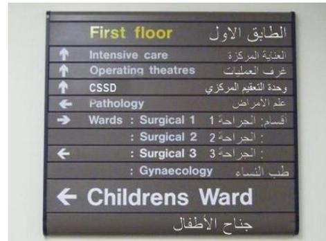
Figure 5.8: Removable slat type signs, with a locking cap
